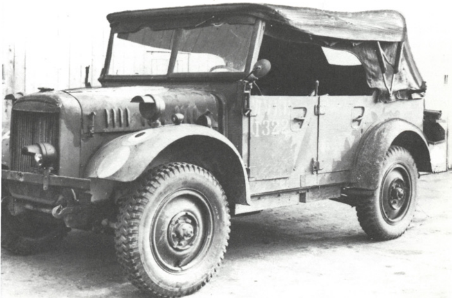
30. Einheits-programme light car, showing typical square bodywork and high ground clearance. This is a captured example with British markings. (STT 6994)
