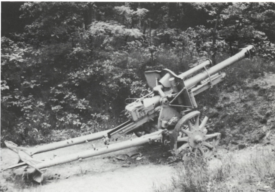
42. Field artillery: a standard late-model 10.5cm gun-howitzer leFH 18/40. This example shows clearly the split-trail carriage and muzzle brake with baffles. (WJKD)
