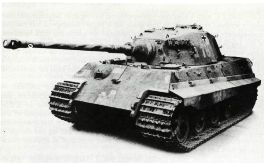
16. The final operational tank, a Tiger 2 ( Koenigstiger ), with the production turret and an 8.8cm L70 gun. Here again the Zimmerit coating and, unusually, a turret cross can be seen. (PC 409)
